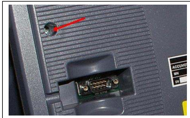
Fig. 3 – Casing is removed quickly and easily with a Phillips-head screw driver. At the time of this writing, removing and replacing the casing leaves no telltale signs.
