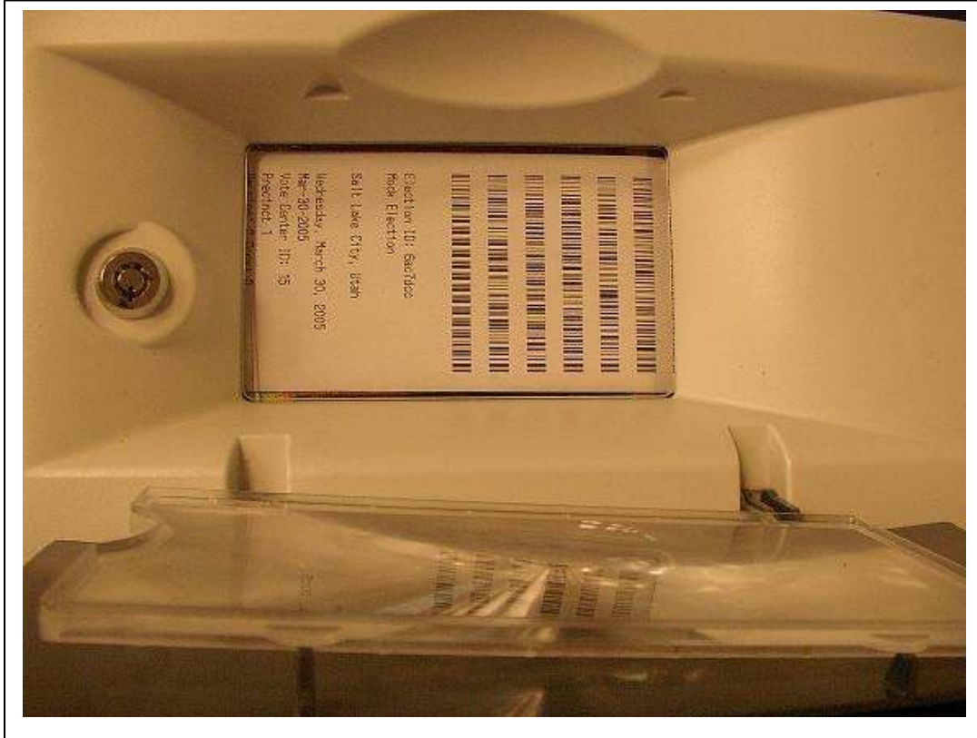
Fig. 15 – Print is small; lower part of paper trail tends not to scroll up into full view.
