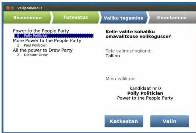
Figure 1: I-voting client — Estonians use special client software and national ID smartcards to cast votes online.
