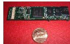
Top left: Cartridge reader/writer prototyped by Hovav Shacham’s research group [7]. Bottom left: Our nonfunctional mockup of installation in cigarette pack. Right: “Gumstix” computer that could be programmed to alter votes in cartridge.
