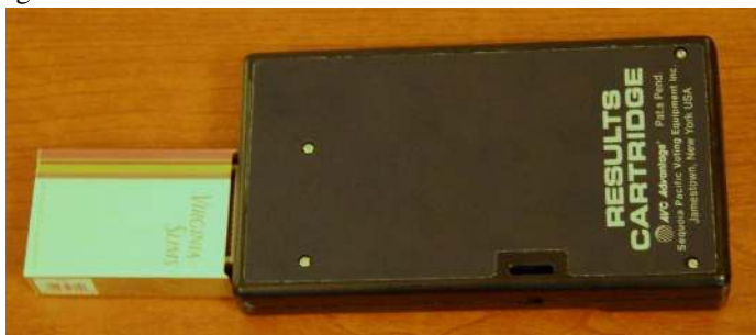
Top left: Cartridge reader/writer prototyped by Hovav Shacham’s research group [7]. Bottom left: Our nonfunctional mockup of installation in cigarette pack. Right: “Gumstix” computer that could be programmed to alter votes in cartridge.
